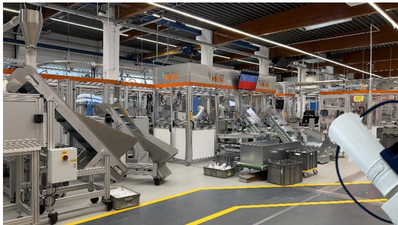
Fully automated Assembly line for drain valves Cycle time 5 sec / part
