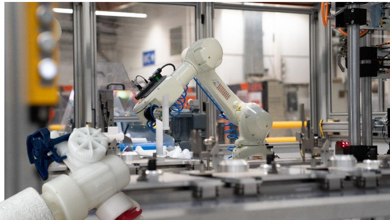
Fully automated Assembly line for inlet valves Cycle time 5 sec / part
