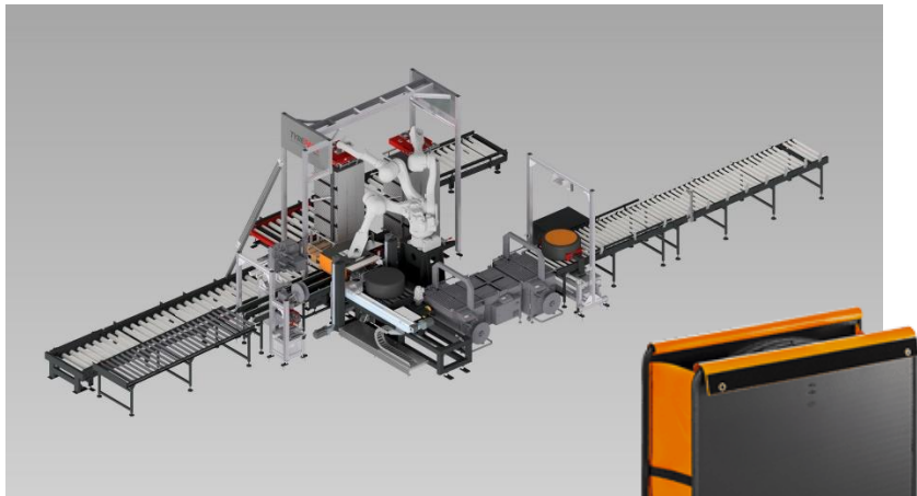
Fully automated packaging of tyres in reuseable packaging Cycle time 12 sec / tyre
