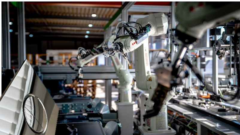
Fully automated Assembly line for push plates Cycle time 4 sec / part
